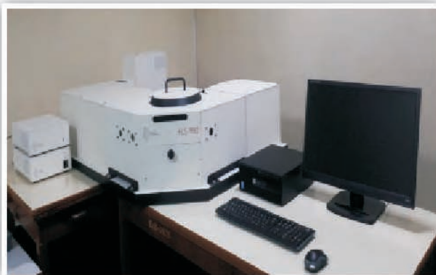
Photoluminescence (PL) measurement setup (F980) from Edinburgh Photonics, UK. This setup can provide PL from 200-800 nm.
