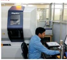
X-Ray Diffraction is a tool used to study the crystal structure of a material or confirm a single phase of a sample. It means XRD is the "finger print" of the material because it identifies which family of crystal structure, the structure of compound belongs to. When X-rays are scattered from a crystalline solid,
