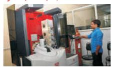
MPMS3 is a brilliant instrument to measure magnetic properties of materials with high accuracy. It employs a SQUID (Super Conducting Quantum Interface Device) detector based technology which can measure very small magnetic fields, just as is observed in a human heart and brain (~10-14 Tesla). It possesses a
